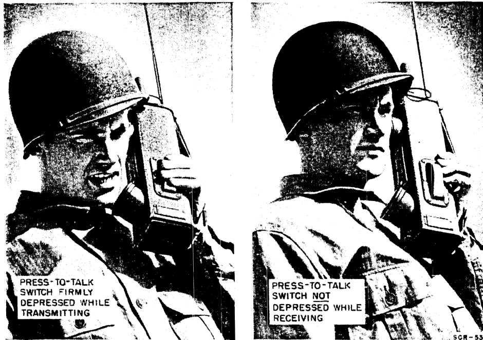
Figure 99. Radio Set SCR-536, showing transmitting and receiving operations.
