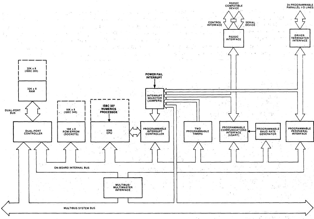
Figure 1. iSBC 86/12A Single Board Computer Block Diagram
