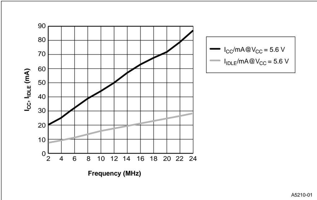
**Figure 1. ICC, IDLE versus Frequency**
